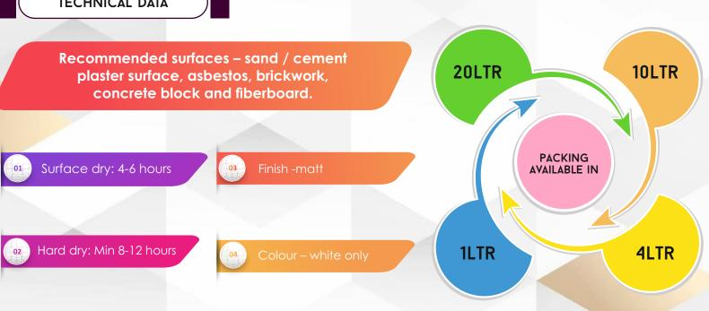
\*it depends on many factors like surface conditions, surface preparation, application skill, weather conditions, dilution etc. The coverage mentioned is under ideal.
